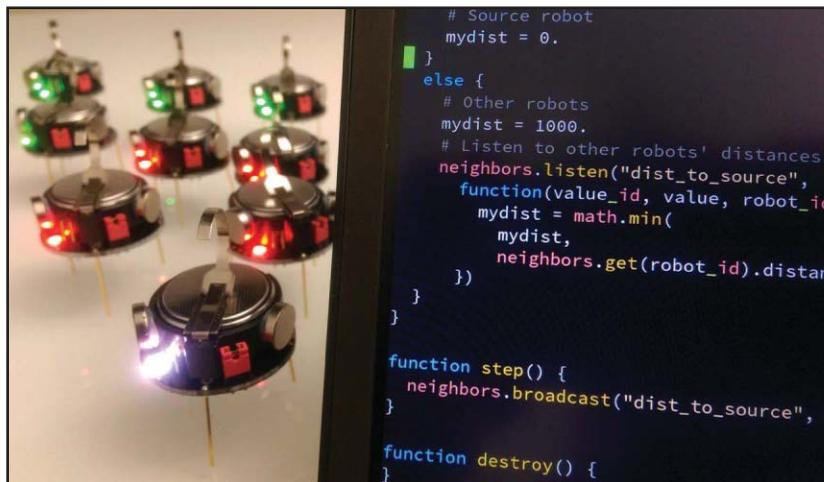
FIGURE 2. Kilobots forming a gradient. The Buzz code for gradient construction is in the foreground.
